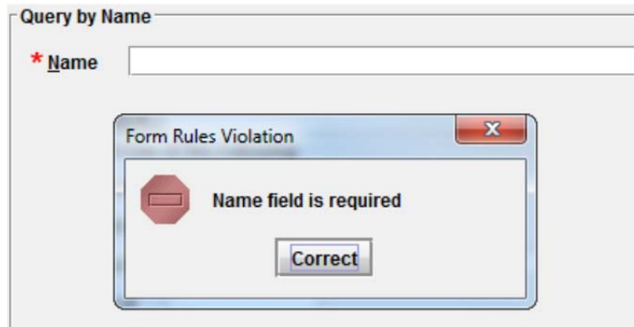
Example of a required field (top) and the error reported if you try to submit the form without filling in a required field (bottom)
