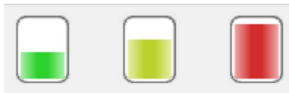
Example of the disk usage display. As more disk space is used to store messages, the icon changes from green (left), to yellow (middle), to red (right)
